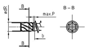
threaded part of the screw b / b2 =  $b_{min}$
