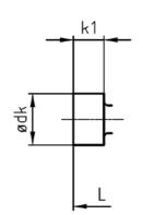
Kombi hexagonal head with thick shaft "SSTA"
